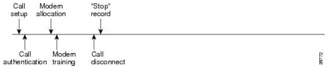
Figure 9 Modem Dial-In Call Setup Sequence With Call Disconnect Occurring Before User Authentication and With Resource Failure Stop Accounting Enabled
