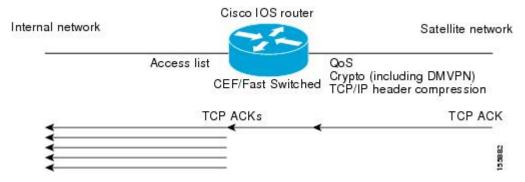
If n ACKs are configured and M is the cumulative ACK point of the original TCP ACK, the resulting TCP ACKs exiting the router will have the following cumulative ACK points:
