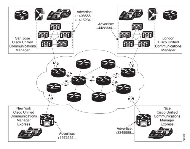
You can configure a Cisco SAF Client either on the same router as the Cisco SAF Forwarder or on an external router.
