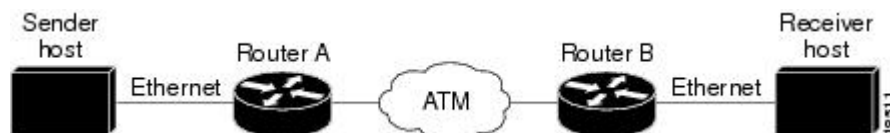
Figure 1 Example RSVP-ATM QoS Interworking Configuration
