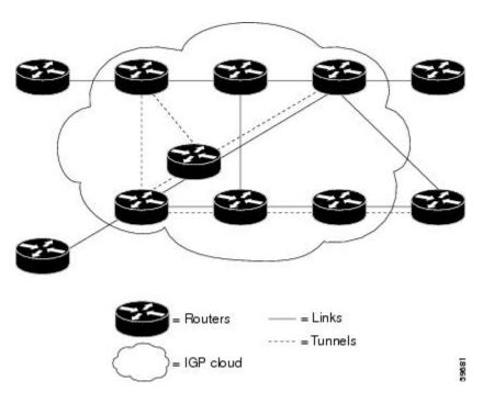
As a result, a TE tunnel is advertised as a link in an IGP network with the link's cost associated with it.
