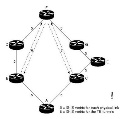
If you have forwarding adjacencies configured on the TE tunnels between B and F and C and F and also on the TE tunnels between F and B and F and C, then when A computes the SPF algorithm, A sees two equal cost paths of 11 to F. As a result, traffic across the A-B and A-C links is shared.
