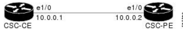
Figure 3 Configuration for Peering with Directly Connected Interfaces Between CSC-PE and CSC-CE Routers
