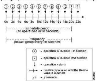
In this example, the first operation (operation 1) in operation group 1 will start at 0 seconds. All 10 operations in operation group 1 (operation 1 to operation 10) must be started in the schedule period of 20 seconds. The start time of each IP SLAs operation is evenly distributed over the schedule period by dividing the schedule period by the number of operations (20 seconds divided by 10 operations). Therefore, each operation will start 2 seconds after the previous operation.
