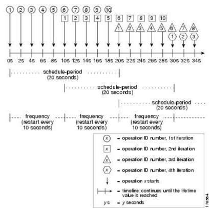
In this example, the first operation (operation 1) in operation group 5 will start at 0 seconds. All 10 operations in operation group 5 (operation 1 to operation 10) must be started in the schedule period of 20 seconds. The start time of each IP SLAs operation is evenly distributed over the schedule period by dividing the schedule period by the number of operations (20 seconds divided by 10 operations). Therefore, each operation will start 2 seconds after the previous operation.
