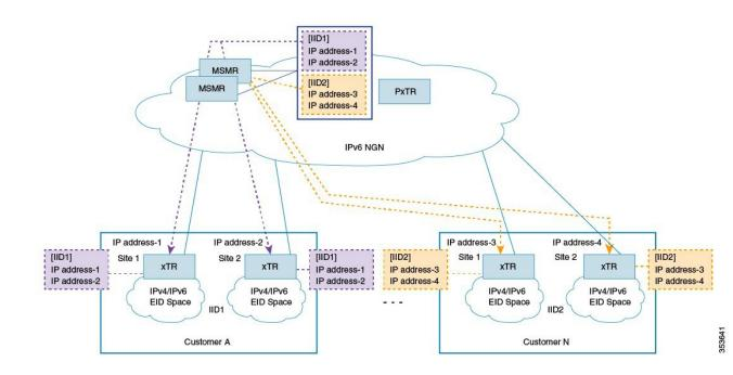
To enable data plane security on the xTRs belonging to customer A (as shown in the image), configure the xTR at site1, as shown below:
