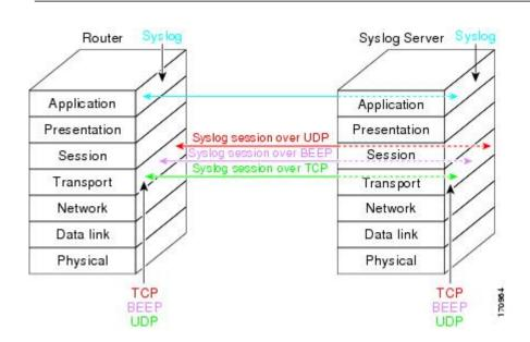
The figure below shows multiple syslog sessions from a single syslog agent to different hosts using UDP, TCP and BEEP.
