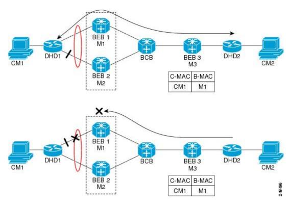
Device DHD1 is dual-homed to two 802.1ah backbone edge bridges (BEB1 and BEB2). Assume that initially the primary path is through BEB1. In this configuration BEB3 learns that the host behind DHD1 (with MAC
