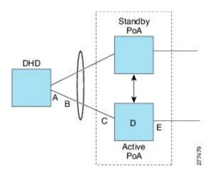
When any of these faults occur, the system reacts by triggering a switchover from the active PoA to the standby PoA. The switchover involves failing over the PoA's uplinks and downlinks simultaneously.
