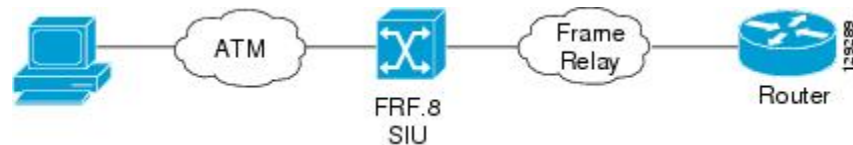
Figure 1: Frame Relay-to-ATM Interworking
