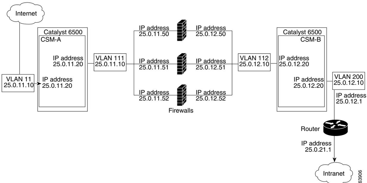
In Figure 13-3, traffic moves through the firewalls and is filtered in both directions. The figure shows only the flow from the Internet to the intranet, and VLANs 11 and 111 are on the same subnet. VLANs 12 and 112 are on the same subnet.
