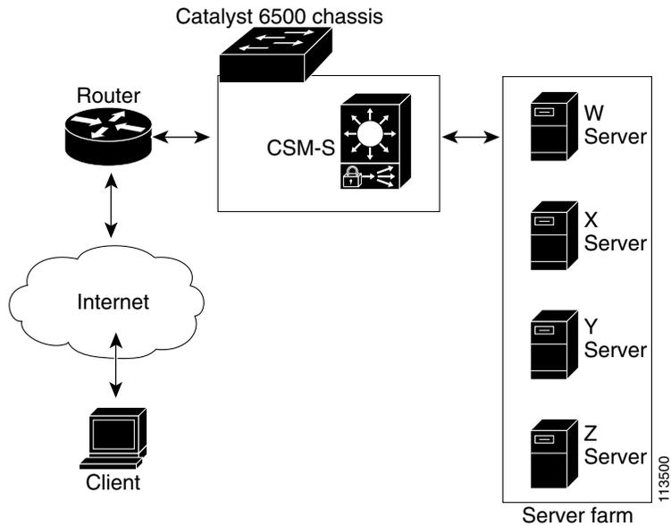
Figure 1-4 describes how the traffic flows between the client and server in a CSM-S environment.
