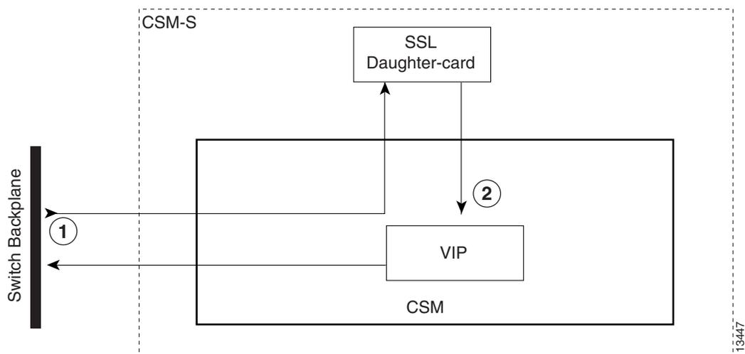
The daughter card runs the SSL software features from SSL releases up to and including SSL release 2.1 supported by Cisco IOS software Release 12.2(18)SXD. See the “Features” section on page 1-2 for a list of supported features for the CSM-S.
