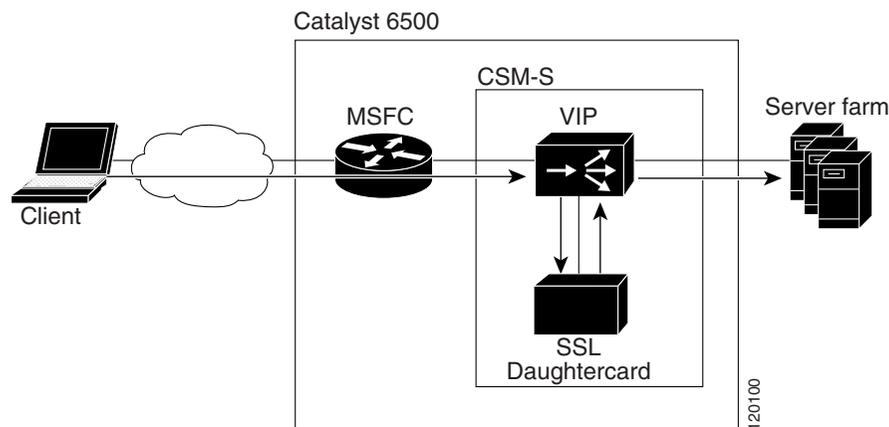
Clients connect to the CSM-S directing their requests to the virtual IP (VIP) address of the virtual server. When a client initiates a connection to the virtual server, the CSM-S chooses a real server (a physical device that is assigned to a server farm) for the connection based on configured load-balancing algorithms and policies (access rules). Policies manage traffic by defining where to send client connections.
