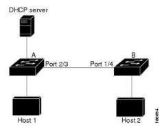
DAI depends on the entries in the DHCP snooping binding database to verify IP-to-MAC address bindings in incoming ARP requests and ARP responses. Make sure to enable DHCP snooping to permit ARP packets that have dynamically-assigned IP addresses.
