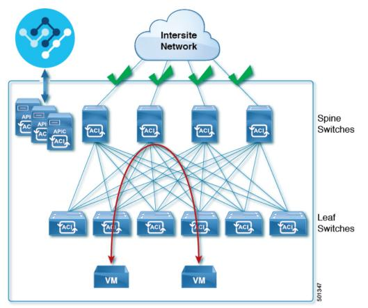
You can choose to mix spine switches supported by Multi-Site with switches that are not supported within the same Cisco APIC fabric, but only the supported switches can connect to the intersite network as shown in the following figure.
