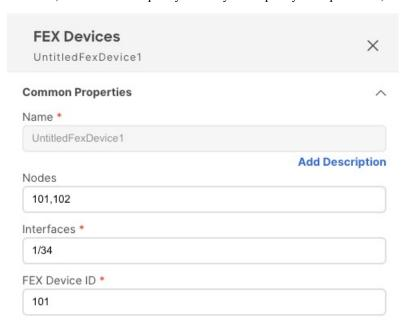
The above configuration means that there are two FEX devices, one connected to leaf switch 101 and another connected to leaf switch 102 with both devices having FEX ID ID 101. Since FEX ID is limited to the leaf switch scope, FEX devices connected to different leaf switches can have the same IDs.
