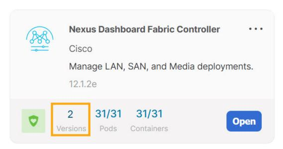
After installation, Nexus Dashboard Fabric Controller service appears in the **Services Catalog**. Note that Versions display as 2 on the Nexus Dashboard Fabric Controller card.
