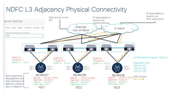
Upgrade or modification from an existing Layer-2 adjacent Nexus Dashboard cluster to a Layer-3 adjacent cluster is not supported. When using Layer 3 adjacency, NDFC service is supported only when the switch connectivity is through the Nexus Dashboard Data interface. Choose NDFC **UI** > **Settings** > **Admin** tab. From the **LAN Device Management Connectivity** drop-down list, select **Data**.
