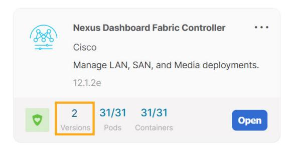
After installation, Nexus Dashboard Fabric Controller service appears in the **Services Catalog**. Note that Versions displays as 2 on the Nexus Dashboard Fabric Controller card.
