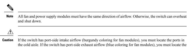
ports in the hot aisle. If you locate the air intake in a hot aisle, the switch can overheat and shut down.
