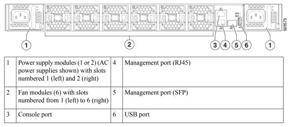
The following figure shows the side of the chassis.
