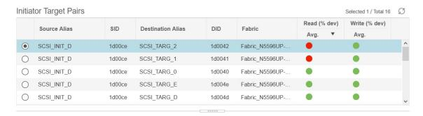
You can click the Status circle icon under **Read** (% **dev**) or **Writer** (% **dev**) columns in the **Initiator-target Pair** table to navigate to the ECT Analysis window, with corresponding Initiator and Target WWPNs prefiltered.
