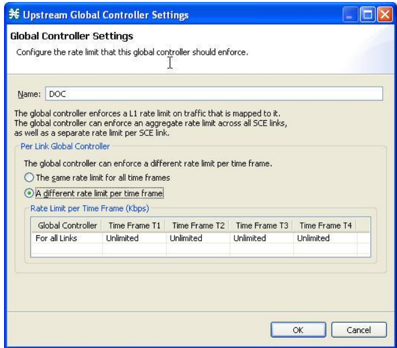
Figure 18: Upstream Global Controller Settings
