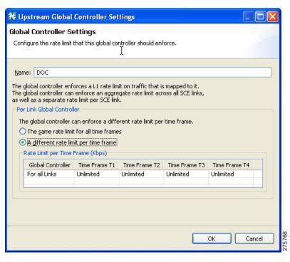
Figure 9-14 Upstream Global Controller Settings
