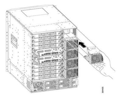
**Step 2** Tighten the captive screws on front left flange of the Fan Module.
