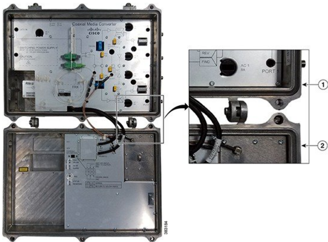
Figure 7: Location of the Waterproof Rubber and EMI Gasket on the Cisco CMC
