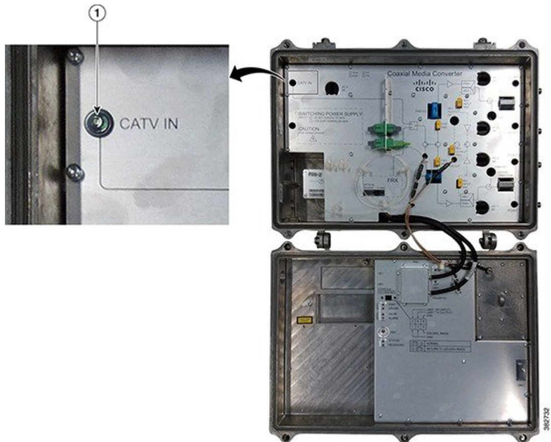
Figure 5: Location of the Seizure Screw
