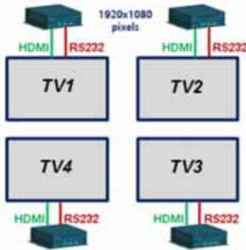
Figure 3 Video Wall with Single DMP Per TV Display
