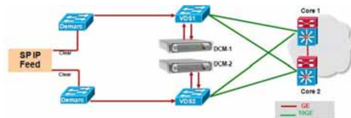
Figure 6 Demarc Connections—Clear IP Feeds
