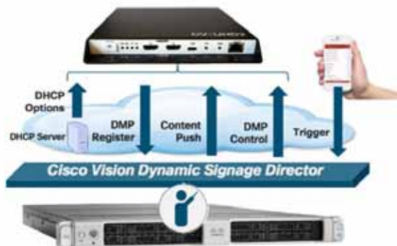
Figure 2 Cisco Vision Dynamic Signage Director Functional Overview
