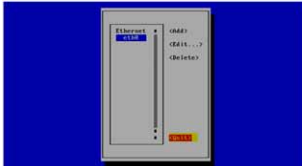
Figure 5 Exit Network Configuration TUI
