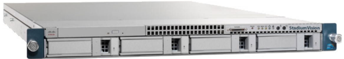
Figure 8 Front Panel of a Cisco StadiumVision Director Platform 2 Server
