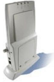
Unlike other Cisco Aironet APs (autonomous APs), the LAPs work in conjunction with the WLC. The WLC manages the AP configurations and firmware.
