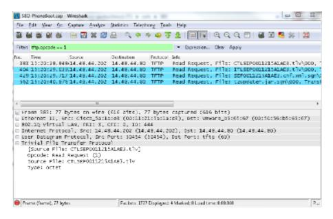
Since the phone received CTL and ITL files from TFTP successfully, the phone asks for a signed configuration file.
