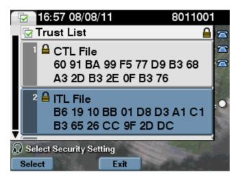
This shows that the MD5sums match. This means that the ITL file on the phone matches the file on the CUCM, so it does not need to be deleted.
