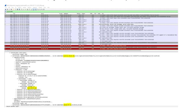
But when we inspect the certificate presented on port 6972, you can see it is a self-signed certificate (Issuer is itself) with CN set up as cucm-EC.steven.lab. The -EC extension gives the indication that this is the ECDSA certificate set up on CUCM.
