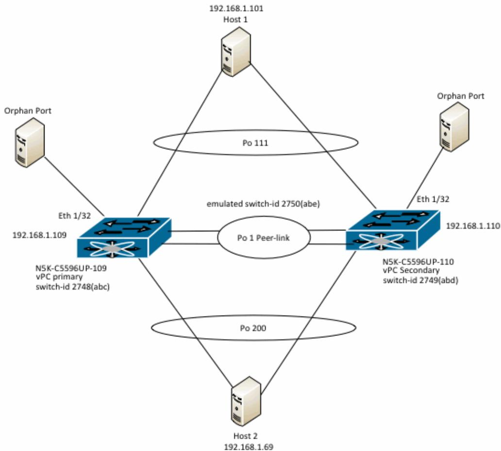
N5K-C5596UP-109 and N5K-C5596UP-110 are a vPC pair of Nexus 5596 switches running NX-OS 5.2(1)N1(2a). N5K-C5596UP-109 is the vPC primary switch and N5K-C5596UP-110 is the vPC secondary
