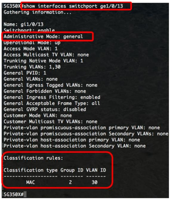
**Note:** In this example, the administrative and operational statuses of interface ge1/0/13 are displayed. The Classification rules table shows that the interface has been mapped to a MAC-based VLAN Group 2 and its traffic will be forwarded to VLAN 30.
