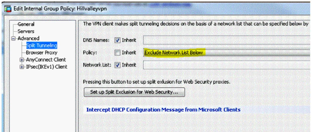
4. Uncheck the **Inherit** box for **Network List** and then click **Manage** in order to launch the Access Control List (ACL) Manager.
