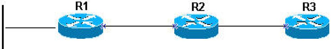
For FEC 10.1.1.0/24, R1 is the Downstream LSR to R2 and R2 is the Downstream LSR to R3.
