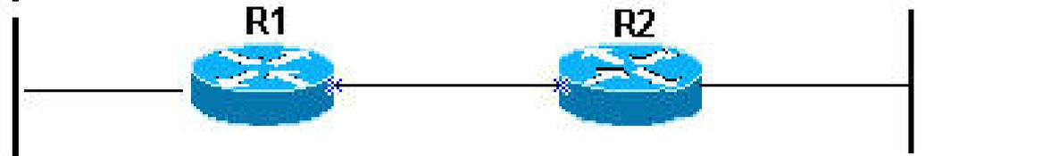
For FEC 10.1.1.0/24, R1 is the Downstream LSR to R2. For FEC 10.2.2.0/24, R2 is the Downstream LSR to R1.
