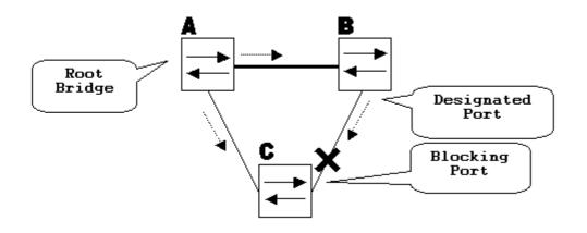
During normal operation, bridge B is a designated port on the link B-C. Bridge B sends BPDUs down to C, which is the blocking the port. The port is blocked while C sees BPDUs from B on that link.
