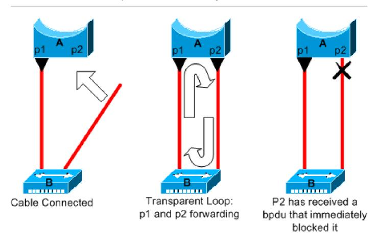
In this example, device A is a bridge with port p1 already forwarding. Port p2 has a PortFast configuration. Device B is a hub. As soon as you plug the second cable into A, port p2 goes to forwarding mode and
