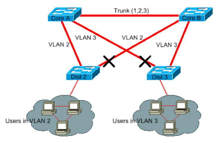
In this design, only one port is blocked per VLAN. Also, with this design, you can remove all redundant links in just one step if you shut down Core A or Core B.
