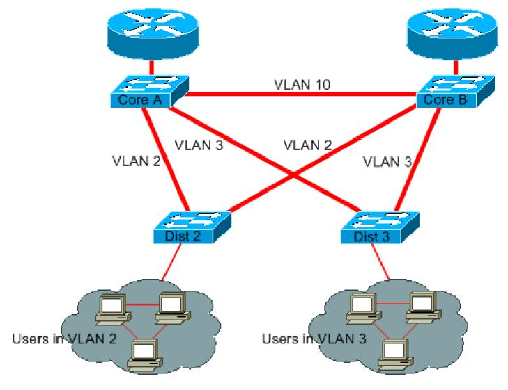
Core A and Core B are now some Layer 3 switches. VLAN 2 and VLAN 3 are no longer bridged between Core A and Core B, so there is no possibility for an STP loop.
