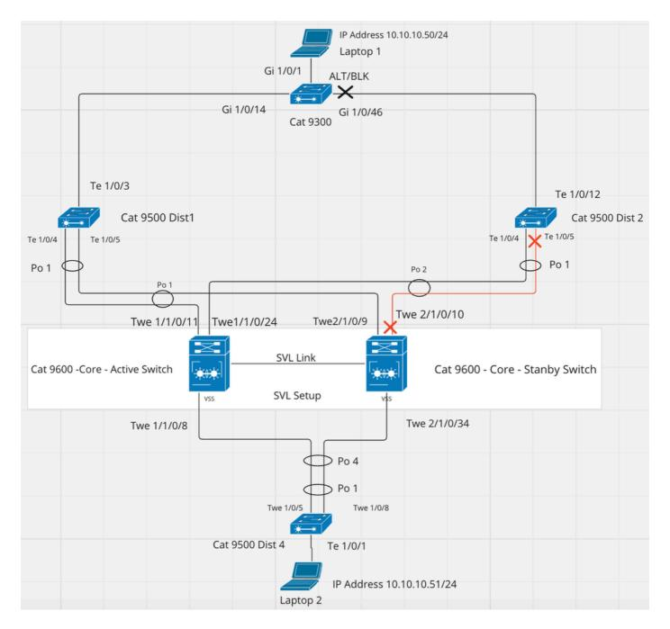
1. Increment of the STP path cost of the port channel between Cat 9600 and Cat 9500 Dist 2 from 10000 to 20000.
