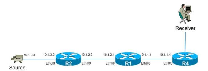
In this example, there is a source with IP address 10.1.3.3 and a receiver for the group 232.1.1.1.
