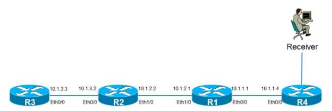
The source **10.1.3.3** is an IP address on the router R3. If you place the command on the Ethernet0/0 interface on the router R1 and ping from the router R3, then the router R1 can reply to the ping. As such, you can perform tests as if there was a directly-connected receiver on the router R1. The **ip igmp join-group** command is placed on the Ethernet0/0 interface on the router R1, and the source is specified in order to ensure
