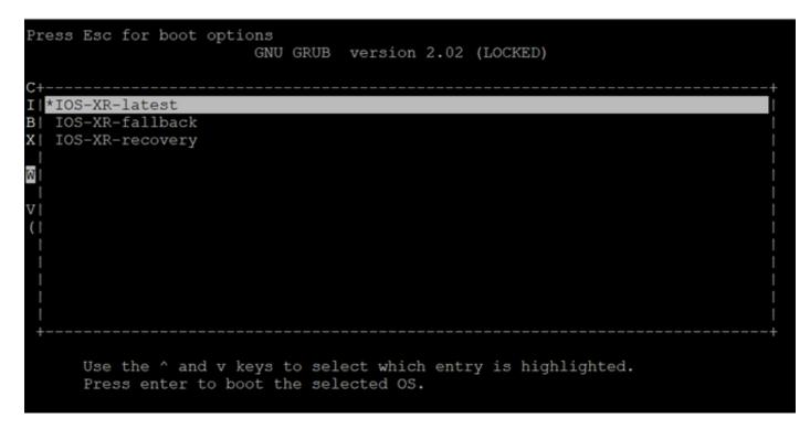
Step 2. On the RP0 card console, select the **IOS XR-recovery** option from the GRUB menu and press **Enter**.
