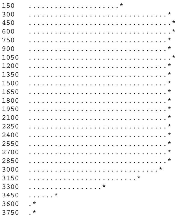
Besides the deeper roll-off at 150 Hz and extinguished frequencies at the high end, it is also typical for ADPCM to expose a lower signal-to-noise ratio (SNR). Though it might still be possible for V.34 modems to use higher symbol rates, it is generally advisable to limit the rate to 2743 baud maximum.
