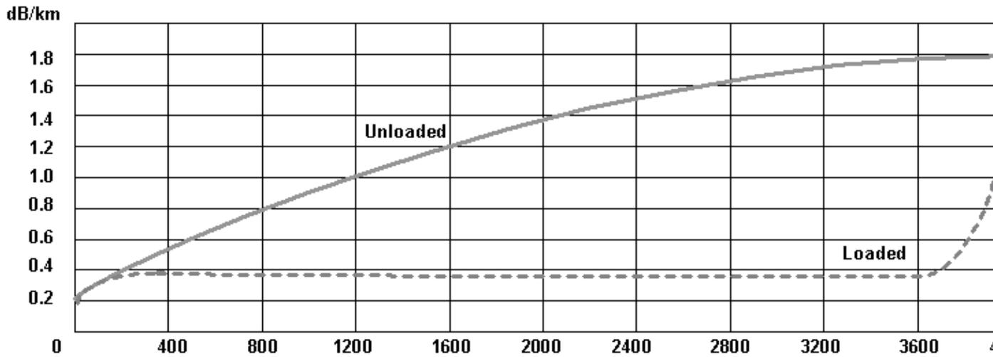
With a load coil, the three-mile loop discussed above reveals a roll-off point at around 3300 Hz only.
