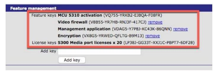
**Note**: Remove MCU Feature keys, select the **Remove** link next to the **Feature key** in this page.
