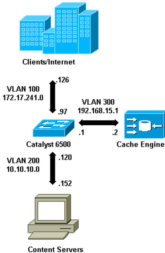
When you install a Cache Engine, Cisco recommends that you configure only the commands necessary to implement WCCP. You can add other features, such as authentication to the router and clients redirection lists, at a later date.
