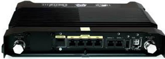
Figure 2. Cisco 829 Industrial Integrated Services Router
