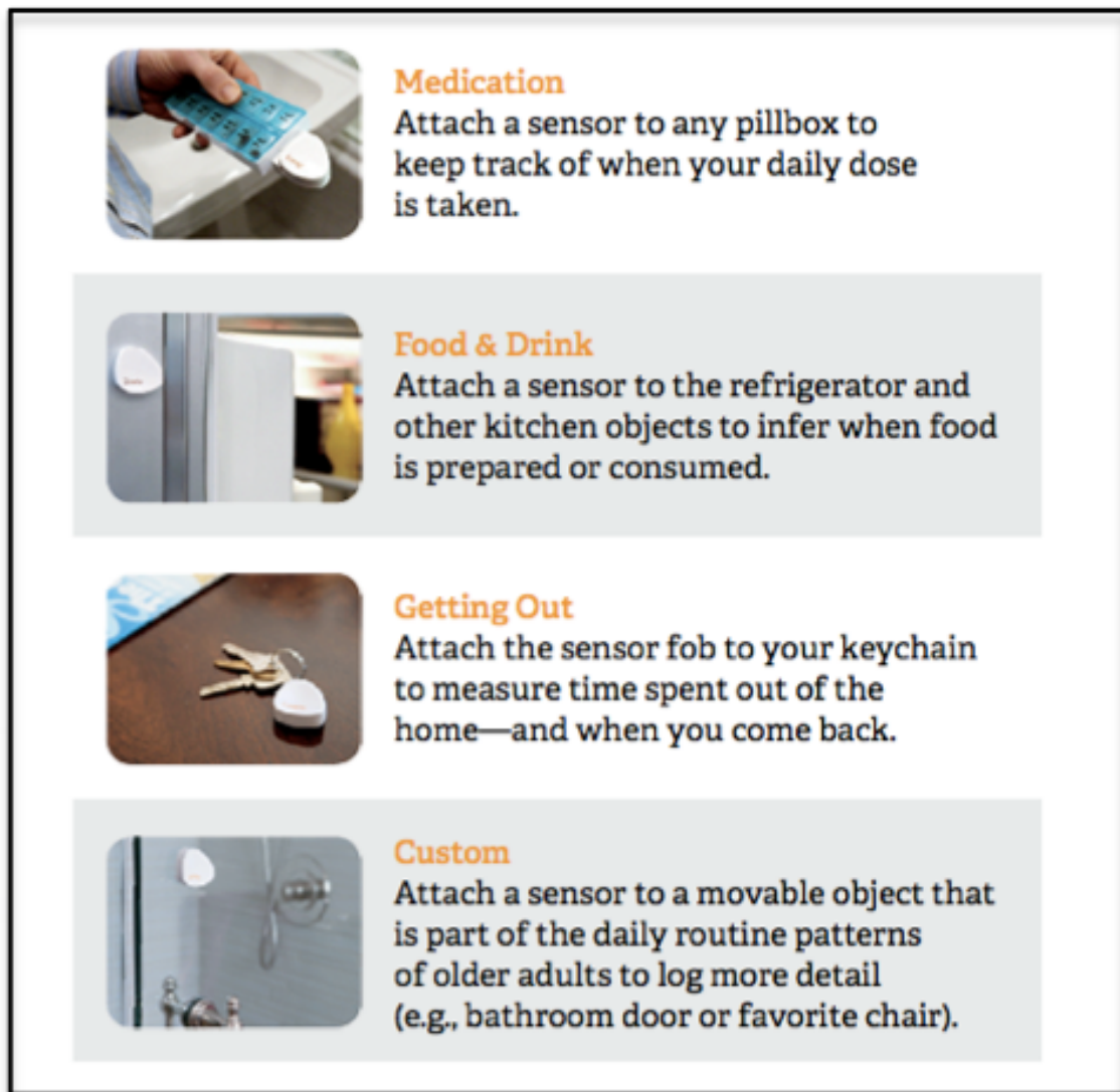
Figure 6. Sensors Placed on Everyday Objects to Monitor Activity 11 (Image source: www.mylively.com)
