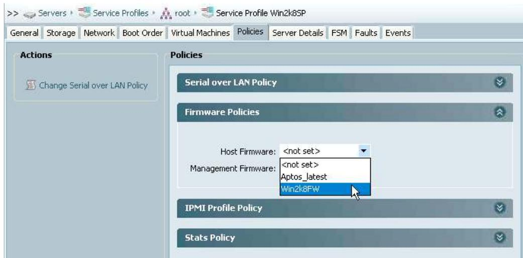
Service profiles in Cisco UCS Manager can be accessed, created, and modified by external management tools using XML APIs. The API also provides integration with external configuration management databases for inventory population, asset tracking, and granular configuration and state information. Since they reside below the operating system, service profiles can be used in conjunction with existing tools, like those for patch management.
