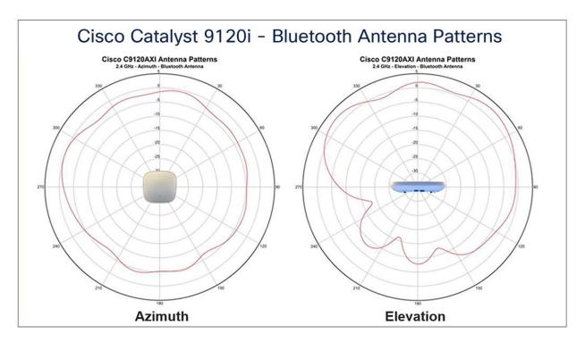
**Figure 1.** Antenna radiation patterns
