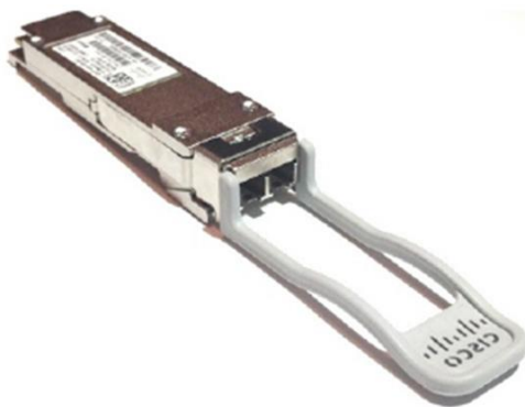
Figure 2. Cisco QSFP BiDi Transceiver (QSFP-40G-SR-BD)
