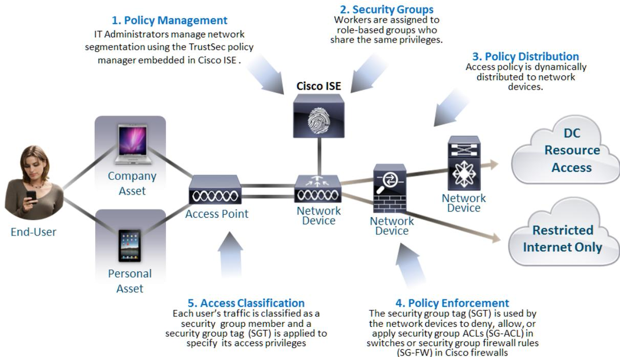
Those centrally defined roles also serve to replace the traditional function of switches in controlling network segmentation. Many organizations that have grown quickly or have legacy infrastructure have run out of possible VLAN capacity in their switches. VLANs have always been defined on each switch to create virtual segmentation between departments, data centers, and functional components of a network.
